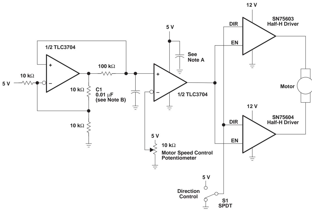
NOTES: A. The recommended minimum capacitance is 10  $\mu\text{F}$  to eliminate common ground switching noise.
