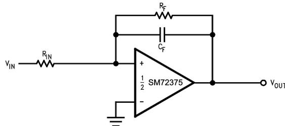
**Figure 25. Canceling the Effect of Input Capacitance**
