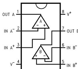
**Figure 1. 8-Pin VSSOP - Top View
