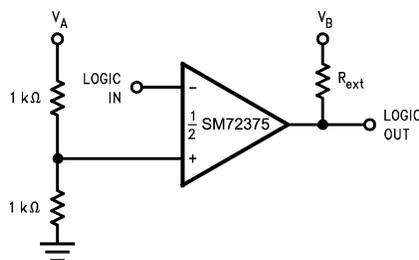
**Figure 26. Universal Logic Level Shifter**
