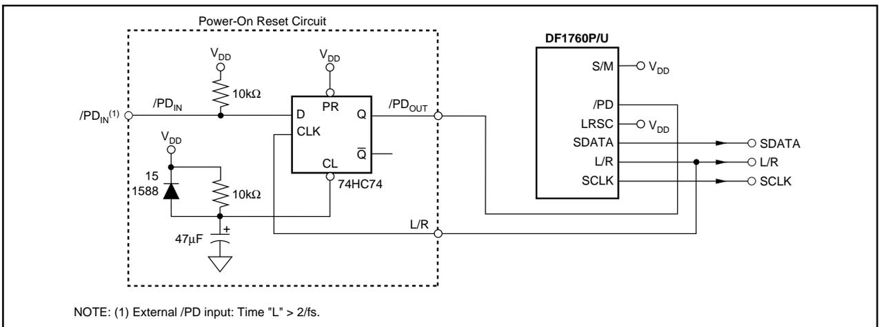
FIGURE 12. Slave Mode Reset Circuit, (LRSC = H).
