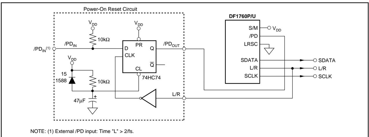
FIGURE 13. Slave Mode Reset Circuit, (LRSC = L).
