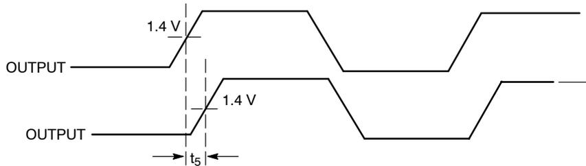
Figure 5. Output-Output Skew
