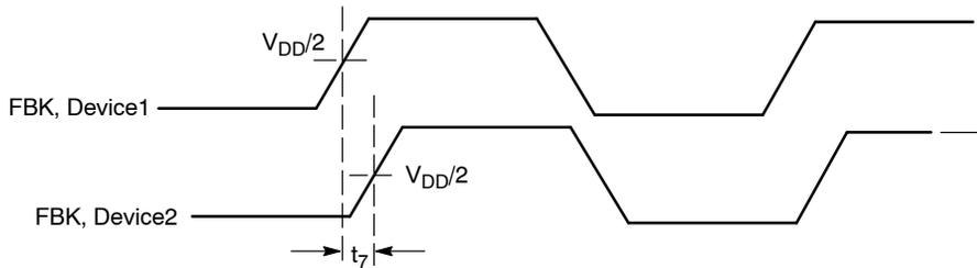
Figure 7. Device-Device Skew
