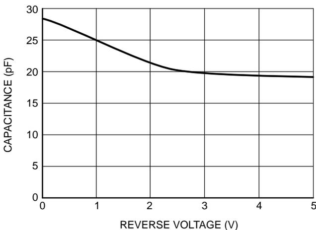
Figure 3. Typical Line Capacitance vs. Reverse Bias Voltage
