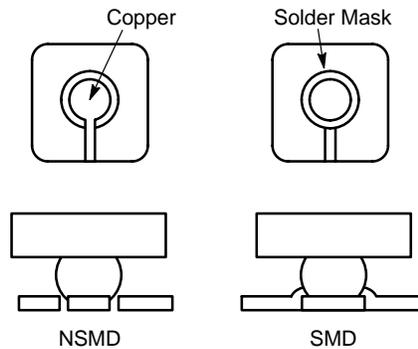
Figure 5. Solder Mask versus Non-Solder Mask Definition
