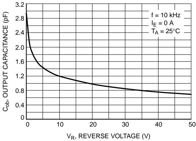
Figure 4. Output Capacitance
