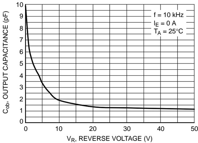
Figure 9. Output Capacitance
