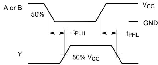
Figure 3. Switching Waveforms
