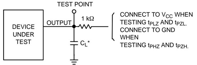
\*Includes all probe and jig capacitance
