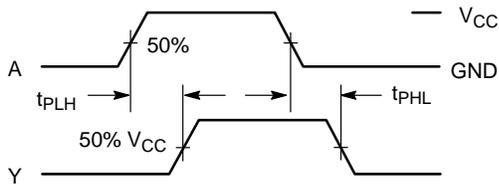
Figure 3. Switching Waveforms
