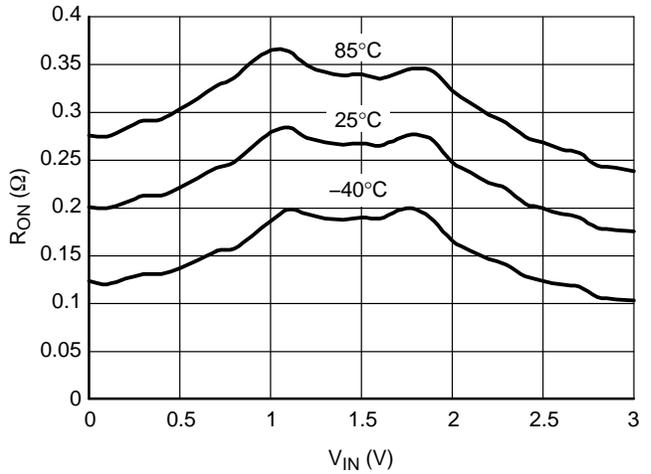
**Figure 10. On-Resistance vs. Input Voltage**
