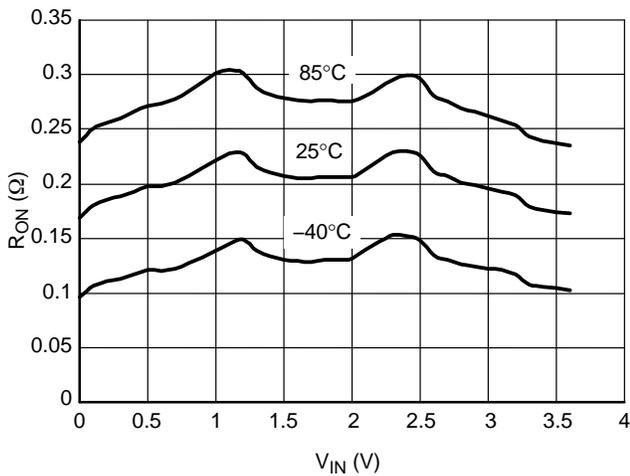
**Figure 11. On-Resistance vs. Input Voltage**
