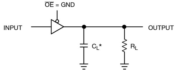
\*Includes all probe and jig capacitance.
