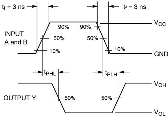
**Figure 3. Switching Waveform**
