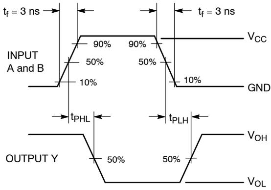
Figure 3. Switching Waveform
