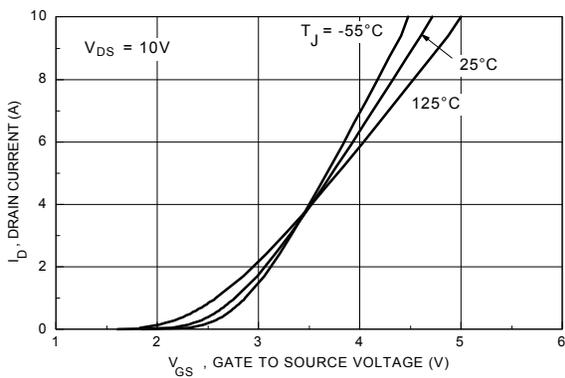
Figure 5. Transfer Characteristics.
