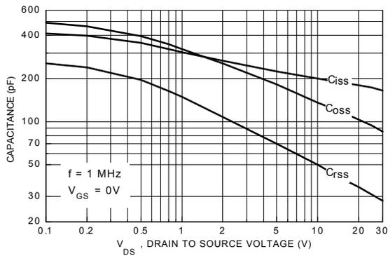
**Figure 9. Capacitance Characteristics.**
