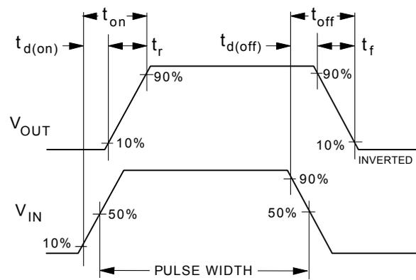
**Figure 12. Switching Waveforms.**
