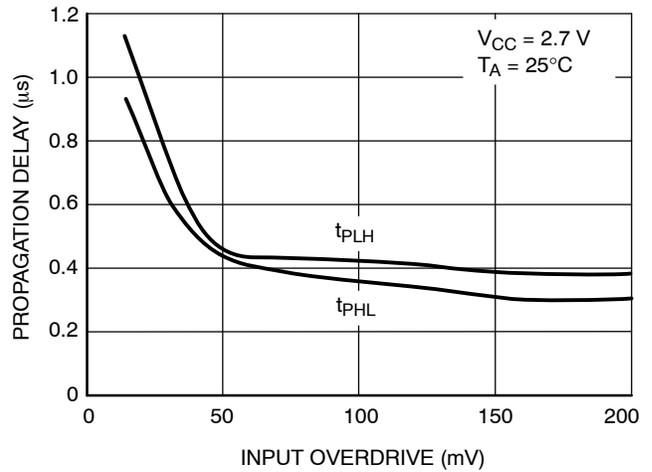
**Figure 10. NCS2200 Series Propagation Delay versus Input Overdrive**
