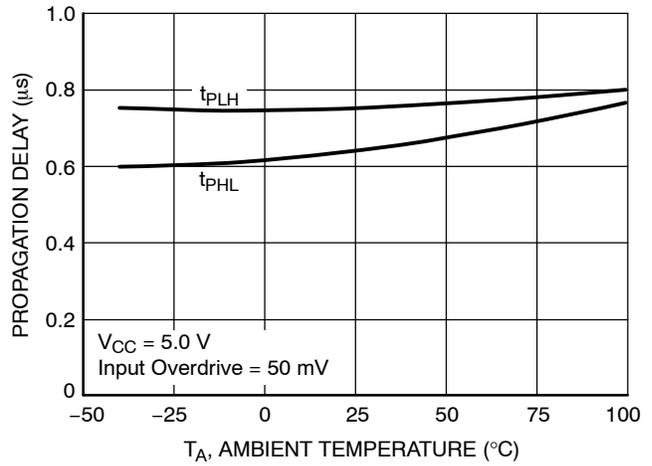
**Figure 8. NCS2200 Series Propagation Delay versus Temperature**
