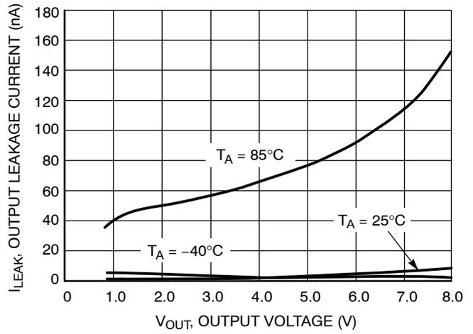
Figure 14. NCS2202 Output Leakage Current versus Output Voltage
