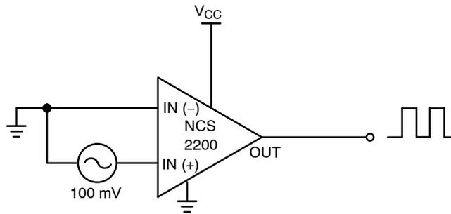
**Figure 20. Zero-Crossing Detector**
