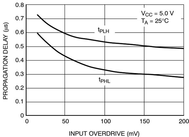
**Figure 11. NCS2200 Series Propagation Delay versus Input Overdrive**
