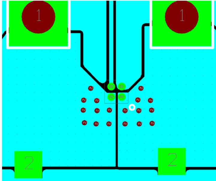
Figure 9. Routing Example 1 oz, 2 Layers, 100 $^{\circ}C/W$
