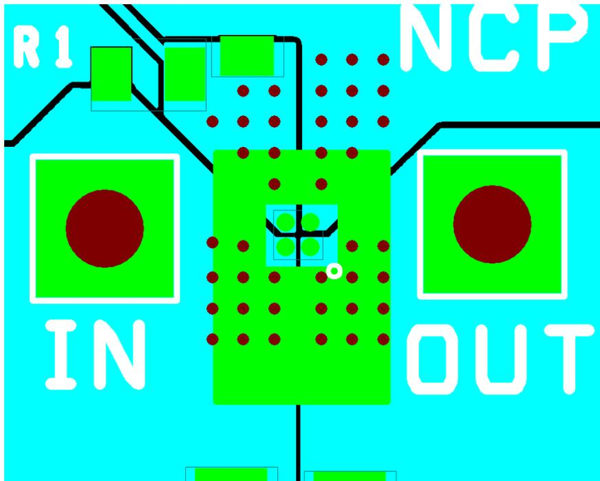
Figure 10. Routing Example 2 oz, 4 Layers, 60°C/W
