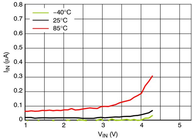
Figure 7. Standby Current (μA) vs V<sub>IN</sub> (V), In Temperature
