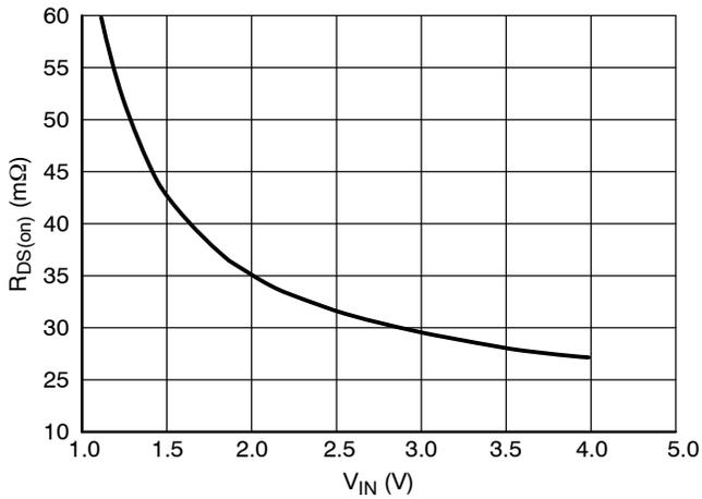
Figure 4. R<sub>DS(on)</sub> (mΩ) vs V<sub>IN</sub> (V), No Load
