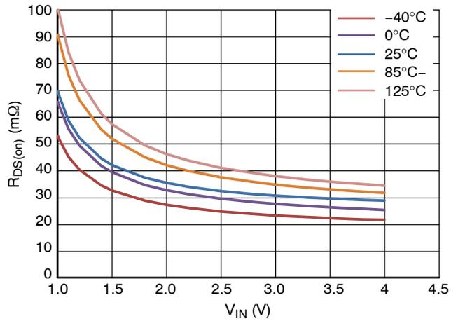
Figure 5. R<sub>DS(on)</sub> (mΩ) vs V<sub>IN</sub> (V) In Temperature (°C), No Load
