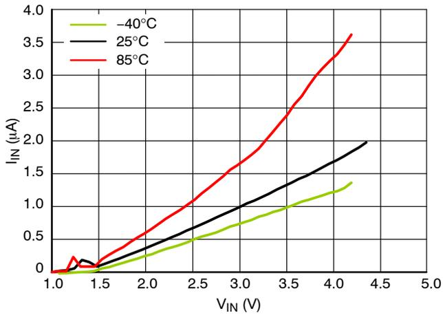
Figure 6. Quiescent Current (μA) vs V<sub>IN</sub> (V), In Temperature
