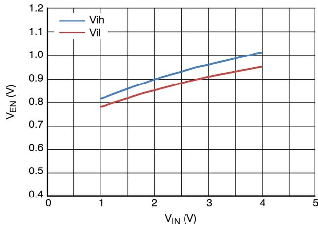
Figure 8. Enable Logic Threshold vs V<sub>IN</sub>
