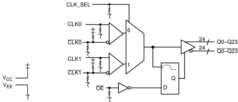
Figure 2. Logic Diagram
