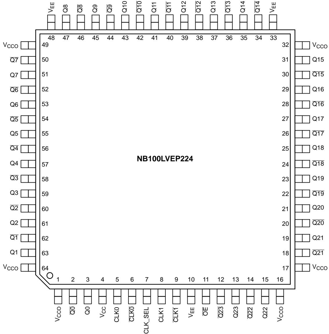
All V<sub>CC</sub>, V<sub>CCO</sub>, and V<sub>EE</sub> pins must be externally connected to appropriate Power Supply to guarantee proper operation. The thermally conductive exposed pad on package bottom (see package case drawing) must be attached to a heat-sinking conduit, capable of transferring 1.2 Watts. This exposed pad is electrically connected to V<sub>EE</sub> internally.
