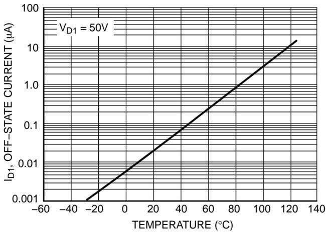
**Figure 1. Typical Off-State Current versus Temperature**
