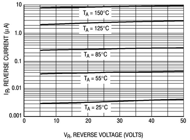
Figure 3. Leakage Current
