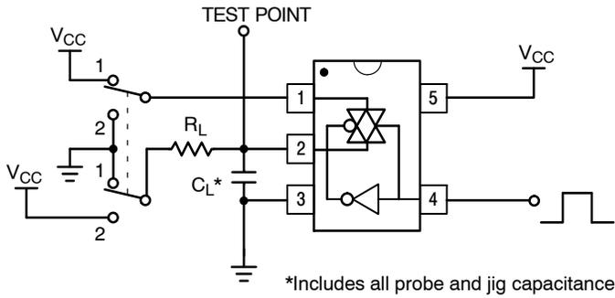
**Figure 8. Propagation Delay Output Enable/Disable Test Set-Up**
