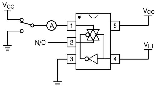
Figure 6. Maximum On-Channel Leakage Current Test Set-Up
