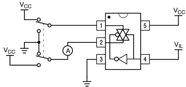
Figure 5. Maximum Off-Channel Leakage Current Test Set-Up
