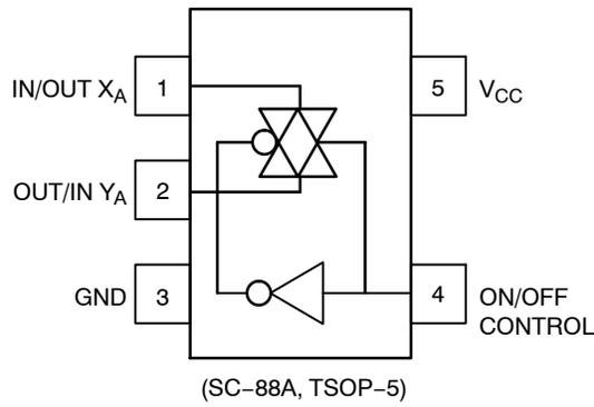
Figure 1. Pinout Diagram
