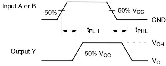
**Figure 4. Switching Waveforms**
