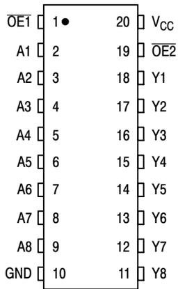
Figure 2. PIN ASSIGNMENT
