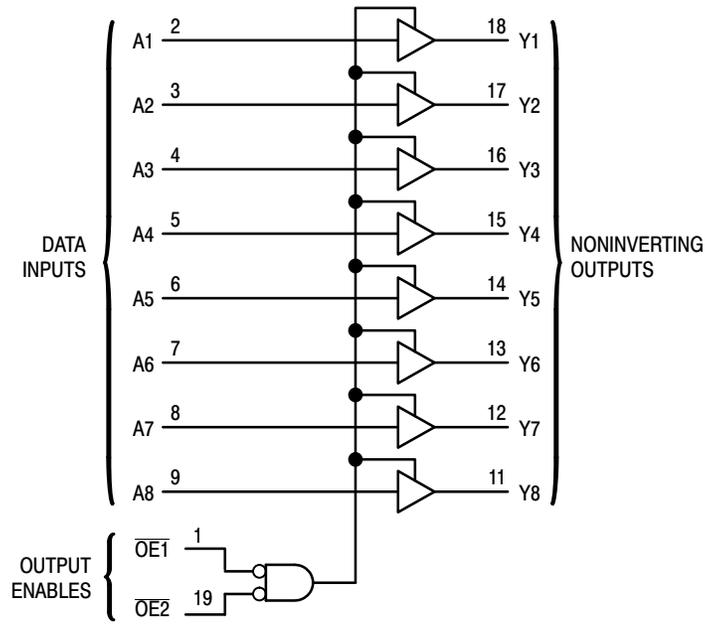
Figure 1. LOGIC DIAGRAM
