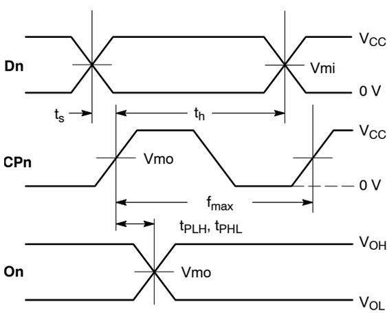
**WAVEFORM 1 - PROPAGATION DELAYS, SETUP AND HOLD TIMES**
