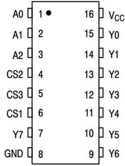
Figure 1. Pin Assignment
