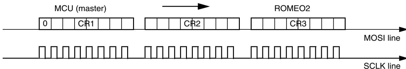
**Figure 13: Reading configuration registers**
