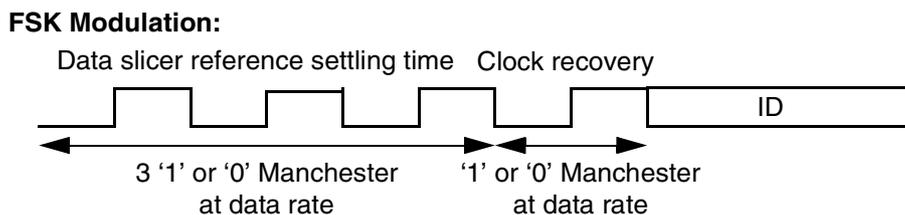
The Header word is a 4 bit Manchester coded message '0110' or its complement sent at the selected data rate. **This bit sequence and its complement must not be found in the sequence preamble and ID word.** Data must follow the Header without any delay.
