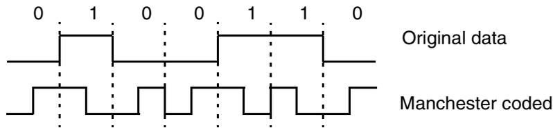
The signal average value is constant. In FSK modulation (MOD=1), clock recovery from the data stream itself is allowed. In order to achieve a correct clock recovery, Manchester coded data must have a duty cycle between 45% and 55%.
