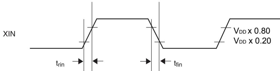
**Note:**  $SR_{IN} = (V_{DD} \times 0.80 - V_{DD} \times 0.20) / t_{rin}$ ,  $SR_{IN} = (V_{DD} \times 0.80 - V_{DD} \times 0.20) / t_{fin}$
