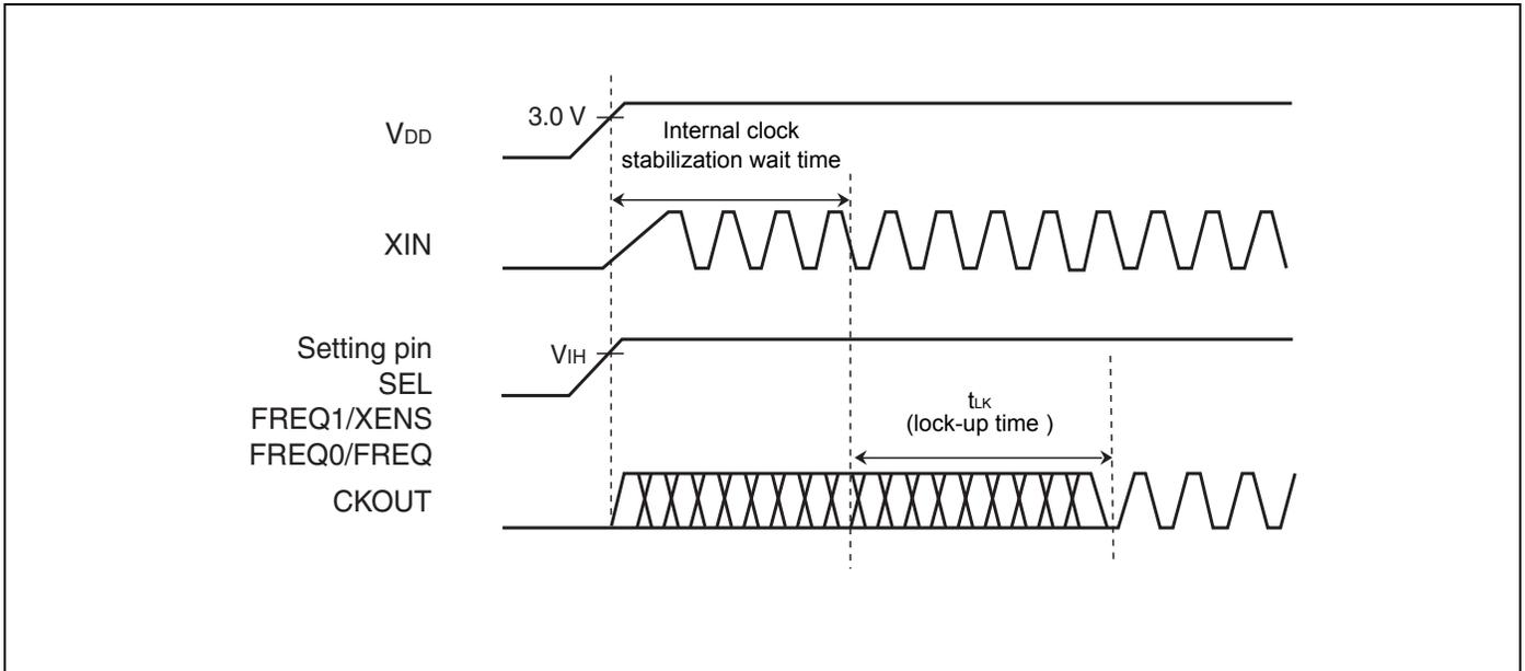
If the setting pin is fixed at the “H” or “L” level, the maximum time after the power is turned on until the set clock signal is output from CKOUT pin is (the stabilization wait time of input clock to XIN pin) + (the lock-up time “ $t_{LK}$ ”). For the input clock stabilization time, check the characteristics of the resonator or oscillator used.
