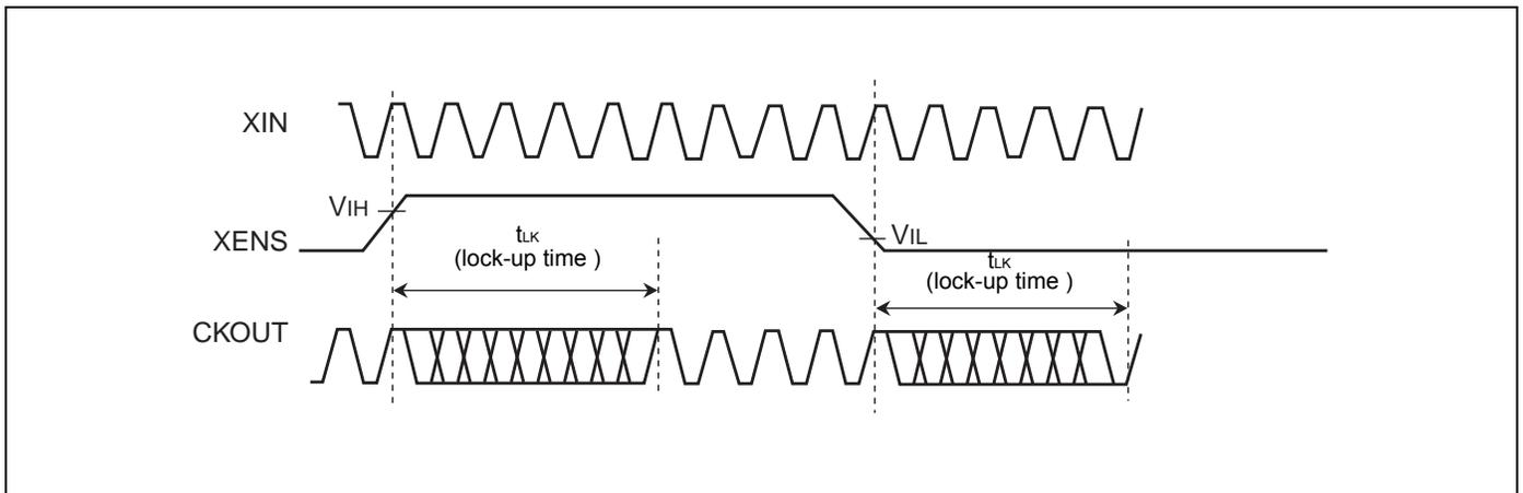
For modulation enable control using the XENS pin during normal operation, the set clock signal is output from CKOUT pin at most the lock-up time ( $t_{LK}$ ) after the level at the XENS pin is determined.
