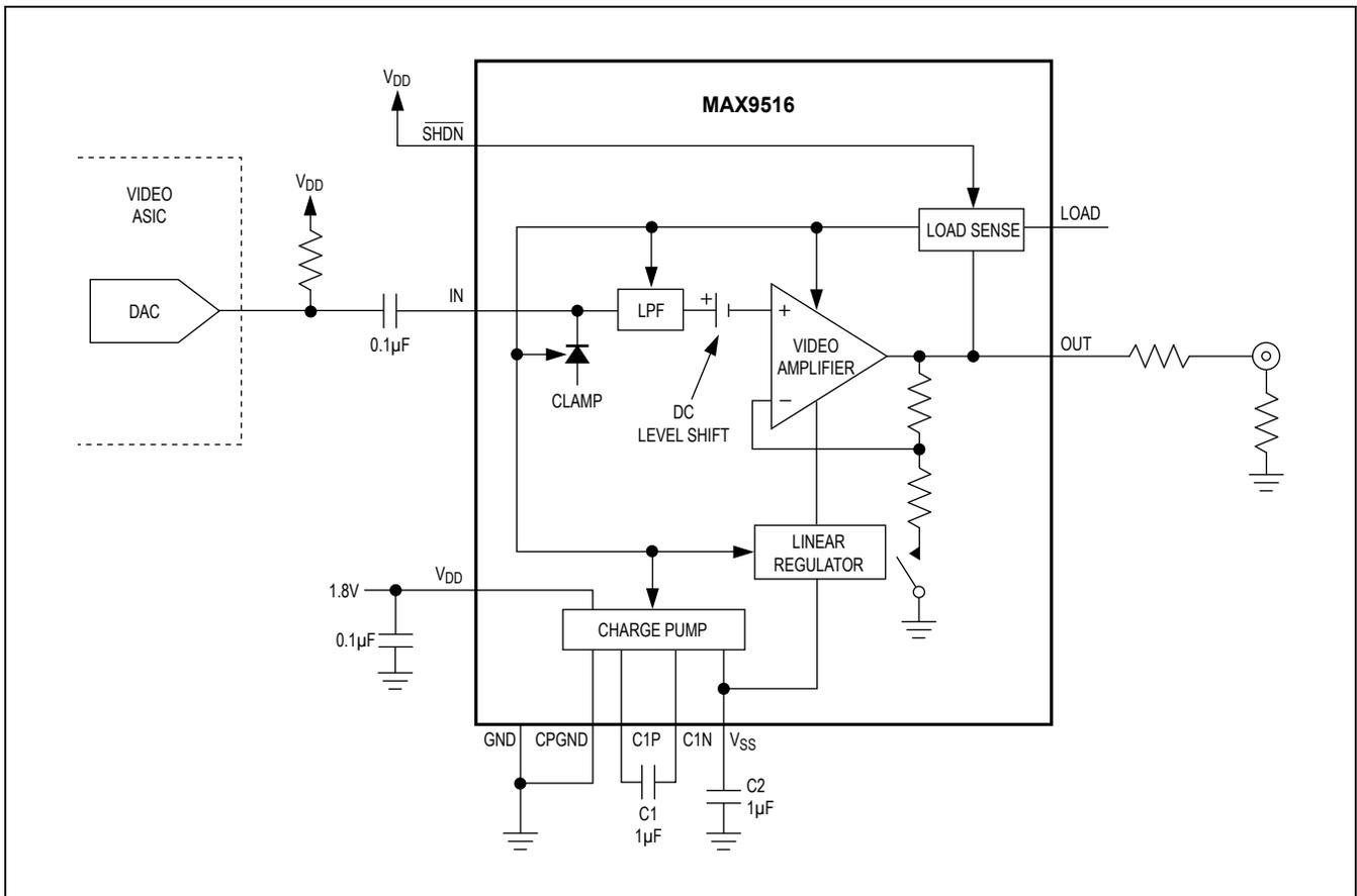
Figure 8. AC-Coupled Input
