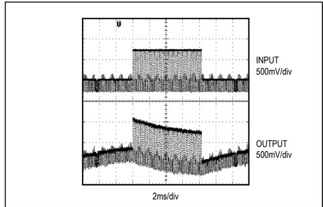
Figure 1. AC-Coupled Output
