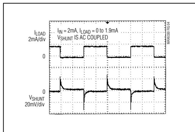
Figure 4. Load-Transient Response with  $C_L = 0.0047\mu\text{F}$
