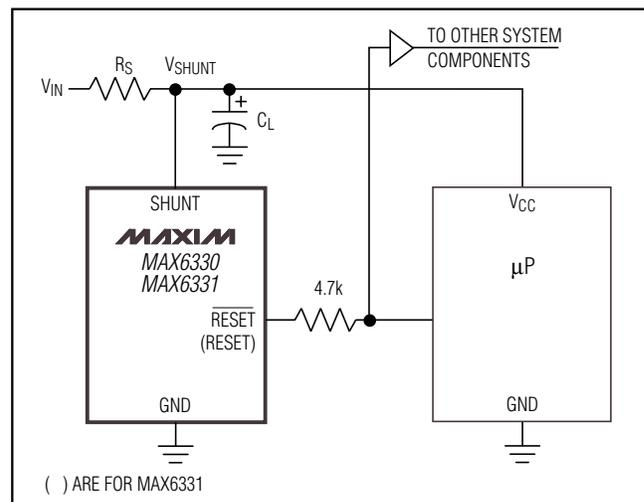
Figure 6. Interfacing to  $\mu\text{Ps}$  with Bidirectional Reset I/O
