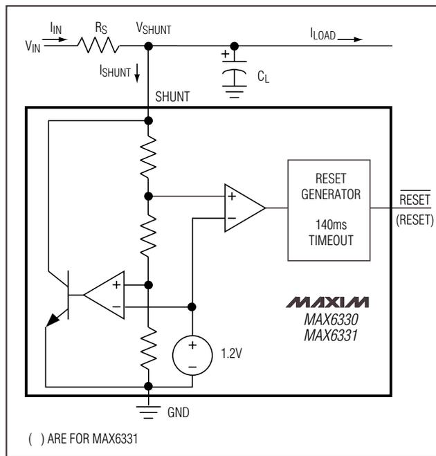
Figure 1. Functional Diagram
