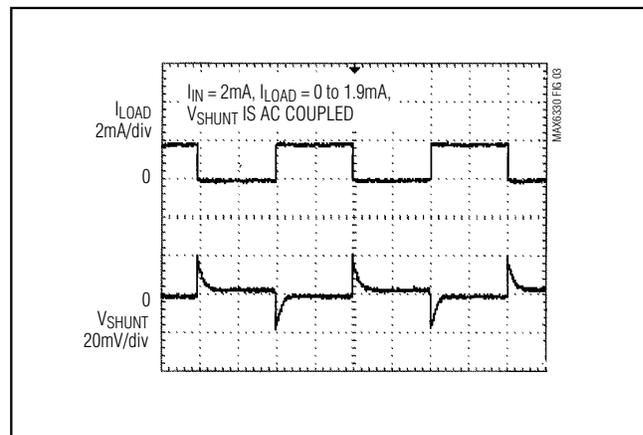
Figure 3. Load-Transient Response with  $C_L = 0.033\mu\text{F}$
