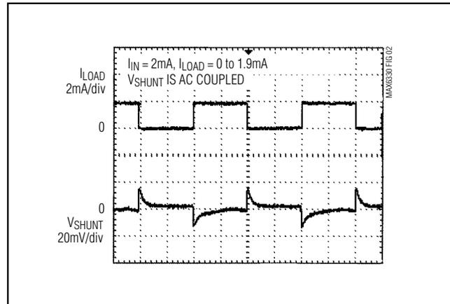
Figure 2. Load-Transient Response with  $C_L = 0.22\mu\text{F}$
