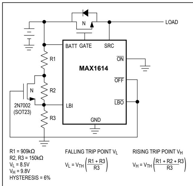
Figure 5. Increasing Hysteresis of the Battery Disconnect Circuit
