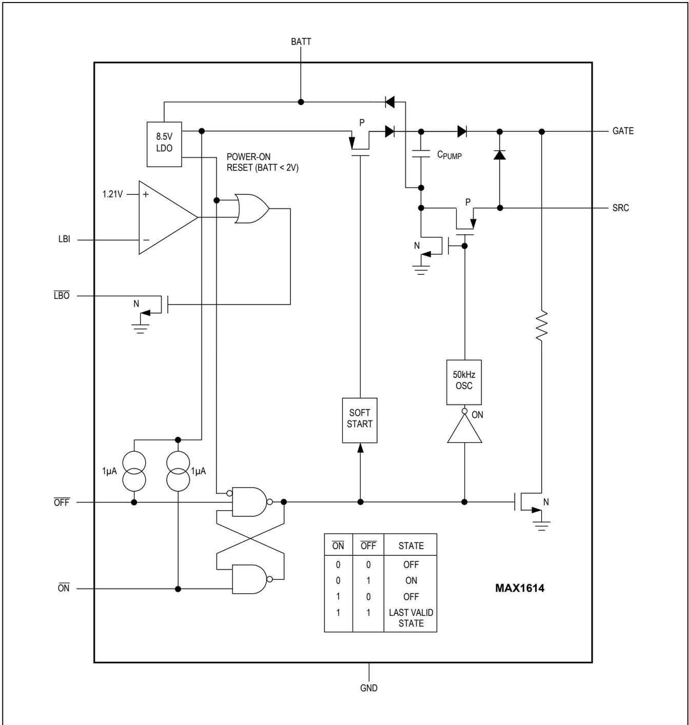
Figure 1. Functional Diagram
