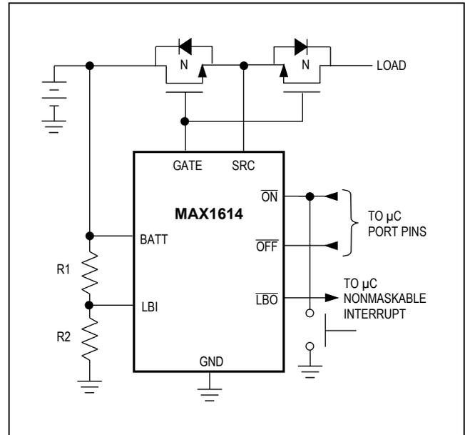
Figure 4. Using  $\overline{\text{LBO}}$  to Generate Early Power-Fail Interrupt
