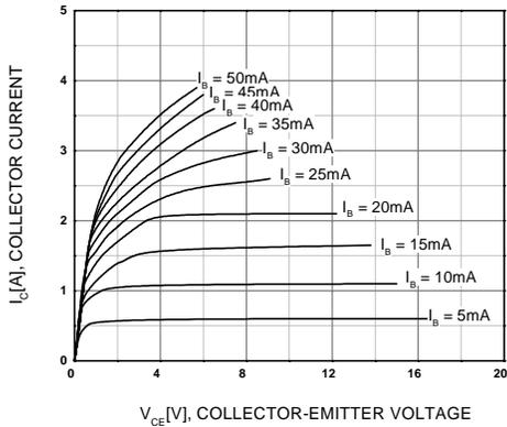
Figure 1. Static Characteristic
