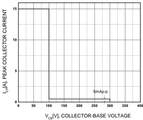
Figure 5. Safe Operating (On Horizontal
