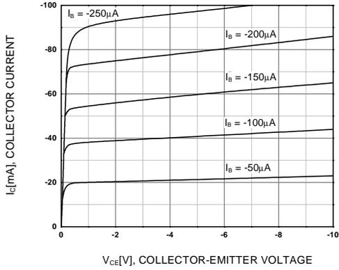
Figure 1. Static Characteristic
