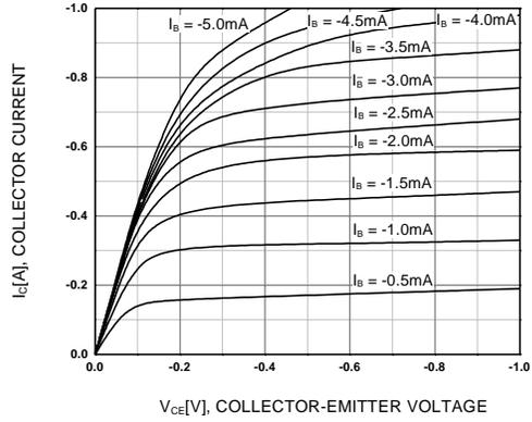
Figure 2. Static Characteristic
