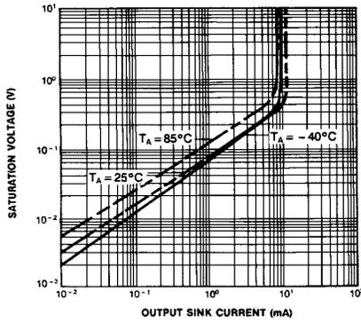
Figure 3. Output Saturation Voltage vs Sink Current
