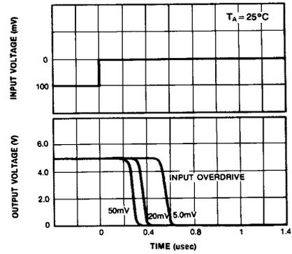
Figure 4. Response Time for Various Input Overdrive-Negative Transition
