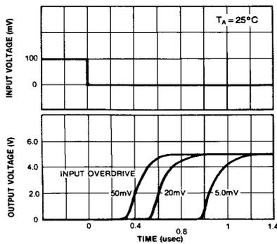
Figure 5. Response Time for Various Input Overdrive-Positive Transition
