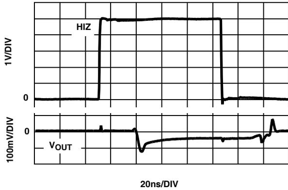
FIGURE 15. HIZ SWITCHING GLITCH  $V_{IN} = 0V$ ,  $R_S = 25$ ,
