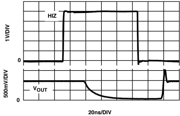
FIGURE 16. HIZ TRANSIENT RESPONSE  $V_{IN} = 1V$ ,  $R_S = 25$ ,
