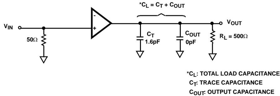
FIGURE 22A. SMALL SIGNAL 200mV<sub>p-p</sub> APPLICATION CIRCUIT
