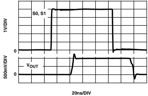
FIGURE 14. CHANNEL TO CHANNEL TRANSIENT RESPONSE
