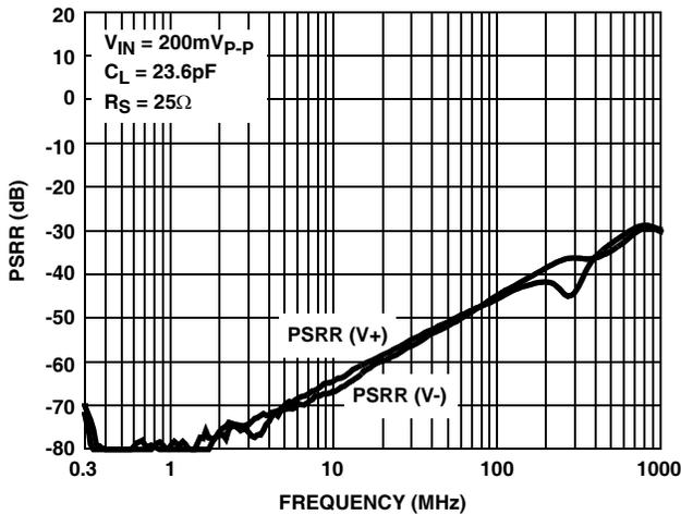
FIGURE 9. PSRR CHANNELS
