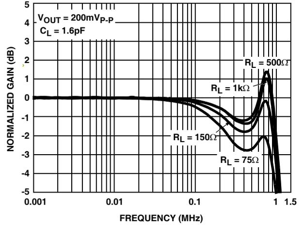
FIGURE 2. SMALL SIGNAL GAIN vs FREQUENCY vs  $R_L$
