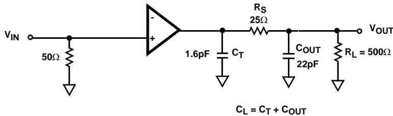
FIGURE 22B. LARGE SIGNAL 1V<sub>p-p</sub> APPLICATION CIRCUIT
