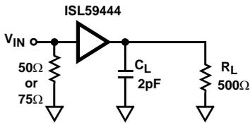
FIGURE 21A. TEST CIRCUIT WITH OPTIMAL OUTPUT LOAD
