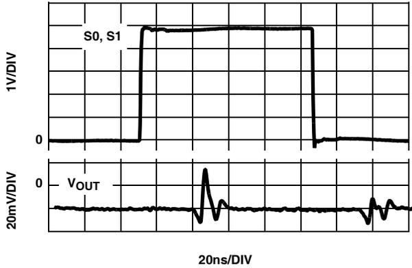
FIGURE 13. CHANNEL TO CHANNEL SWITCHING GLITCH
