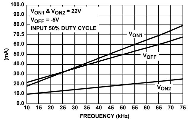
FIGURE 4. SUPPLY CURRENT vs FREQUENCY 8 CHANNELS TOGGLING
