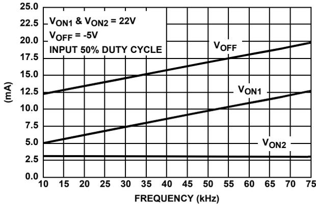
FIGURE 1. SUPPLY CURRENT vs FREQUENCY 1 CHANNEL TOGGLING
