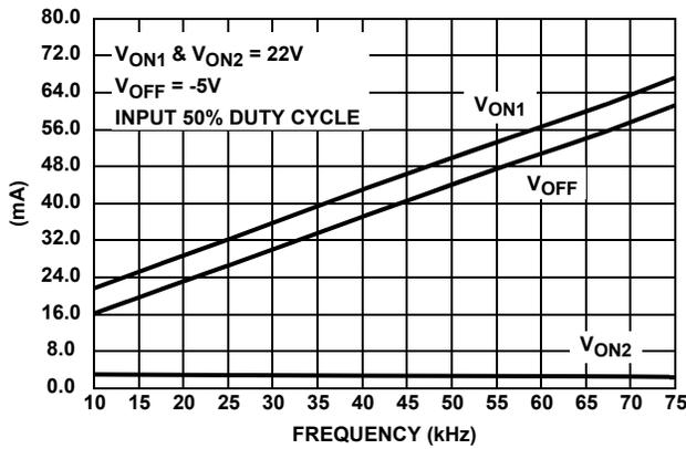
FIGURE 3. SUPPLY CURRENT vs FREQUENCY 6 CHANNELS TOGGLING
