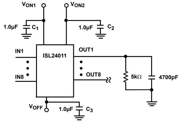
If the output load is a series 200Ω resistor and a 3300pF then C1, C2 and C3 can be reduced to 0.47µF.
