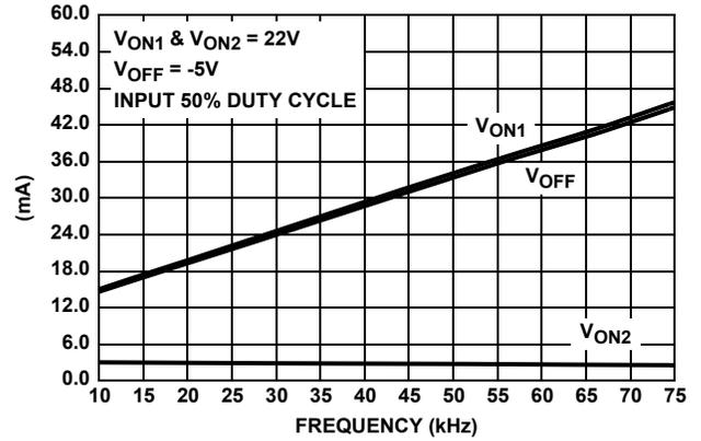
FIGURE 2. SUPPLY CURRENT vs FREQUENCY 4 CHANNELS TOGGLING
