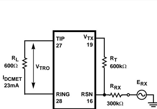
FIGURE 1. OVERLOAD LEVEL (TWO-WIRE PORT)
