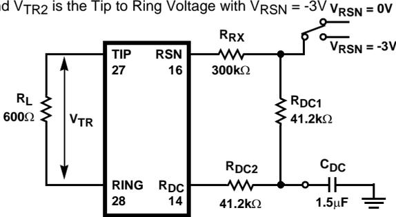
FIGURE 8. CURRENT GAIN-RSN TO METALLIC
