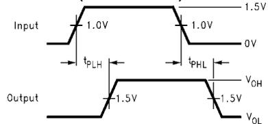
All input pulses have the following characteristics: frequency = 10 MHz,  $t_r = t_f = 2$  ns,  $Z_O = 50\Omega$ . The outputs are measured one at a time with one transition per measurement.
