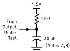
$C_L$  includes probes and jig capacitance. For B Port outputs,  $C_L = 30$  pF is used for worst case edge rate.
