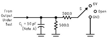
$C_L$  includes probes and jig capacitance.
