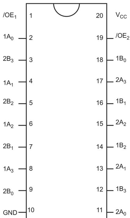
Figure 2. Pin Configuration
