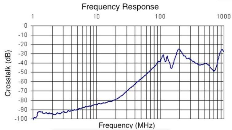
Figure 6. Crosstalk ( $V_{BAIS}=0.5V$ ,  $V_{CC}=3.0V$ ,  $SEL_n=HIGH$ )
