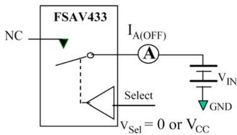
**Figure 9. Off Leakage**
