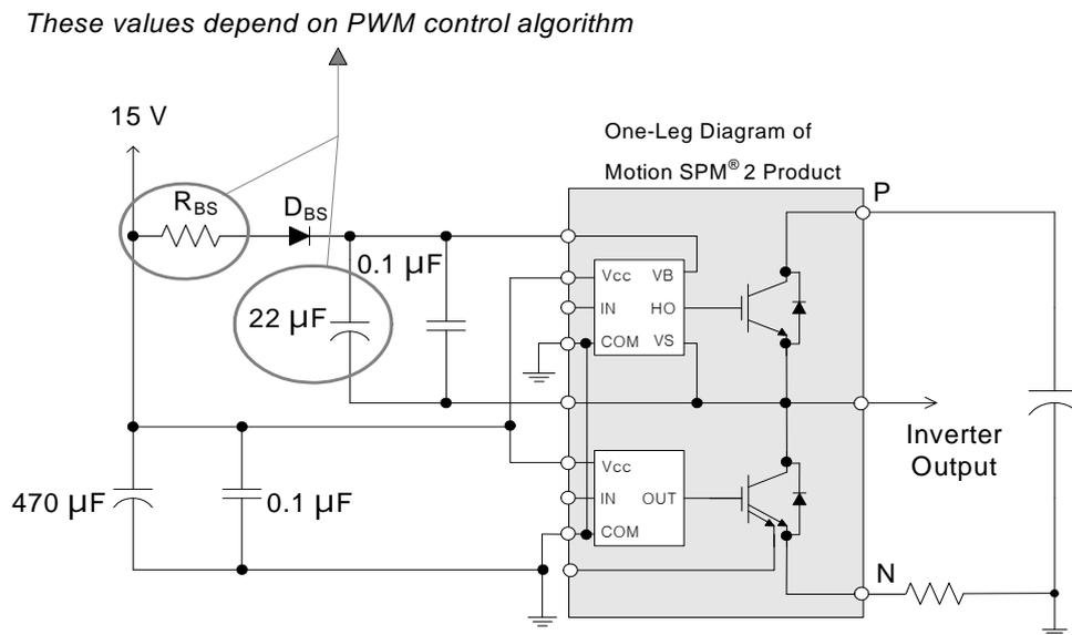
**Figure 13. Recommended Bootstrap Operation Circuit and Parameters**
