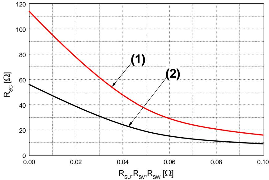
**Figure 6.  $R_{sc}$  Variation by Change of Shunt Resistors ( $R_{SU}, R_{SV}, R_{SW}$ ) for Short-Circuit Protection**
