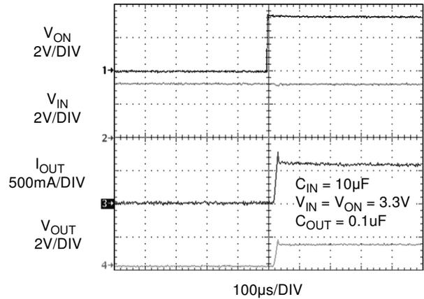
Figure 20. Current Limit Response Time (Output is loaded by 2.2Ω, C<sub>OUT</sub> = 0.1µF)
