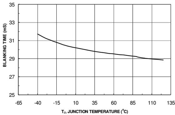
Figure 15.  $T_{BLANK}$  vs. Temperature
