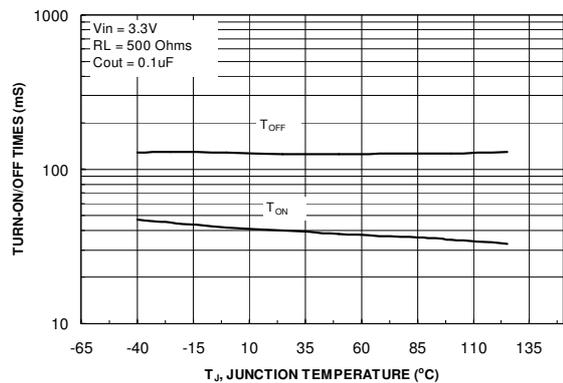
Figure 12.  $T_{ON} / T_{OFF}$  vs. Temperature
