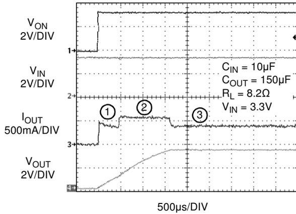
Figure 25. Switch is turned on into a large output capacitor
