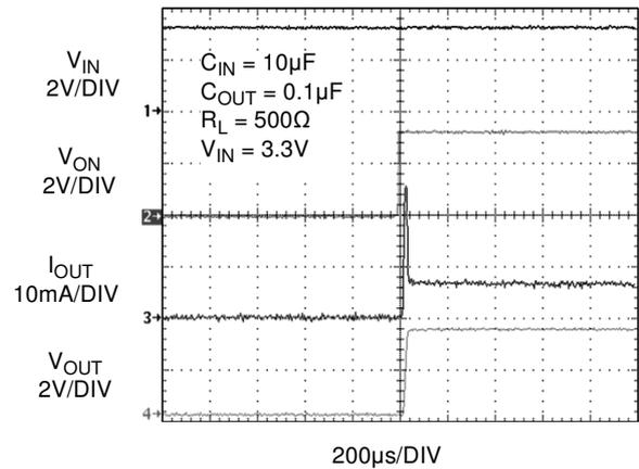
Figure 16.  $T_{ON}$  Response
