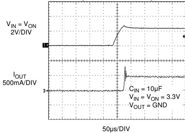
Figure 19. Current Limit Response Time (Switch is powered to a short)
