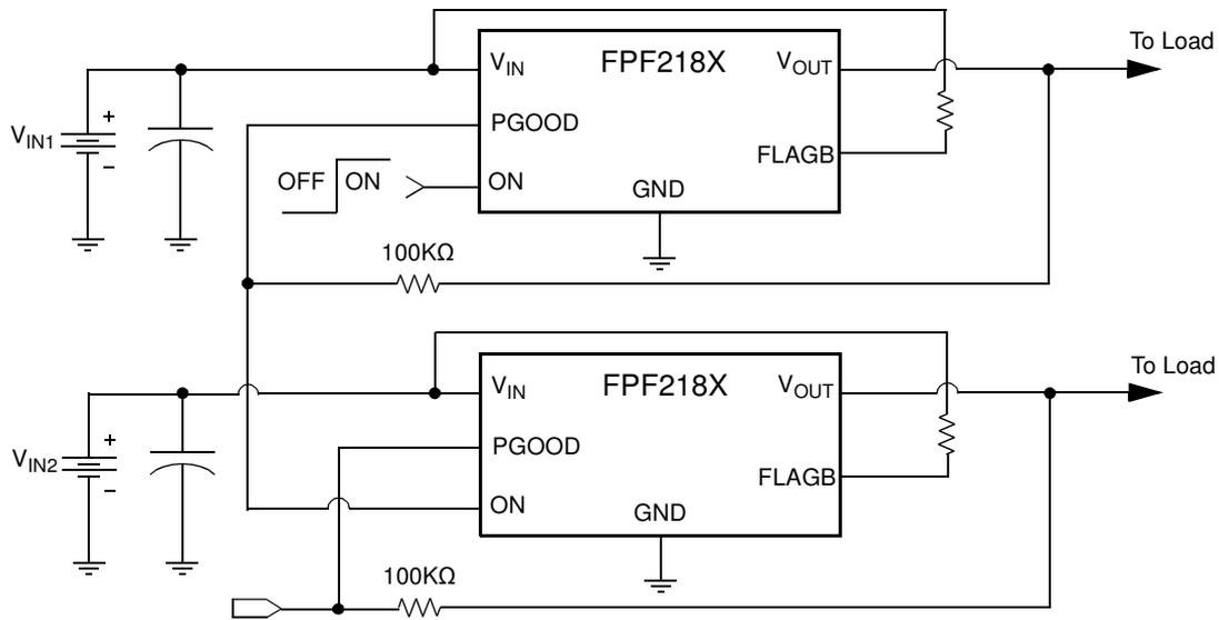
Power good function in sequential startup. No battery is loaded to the output
