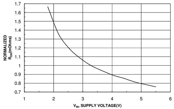
Figure 10.  $R_{ON}$  vs.  $V_{IN}$
