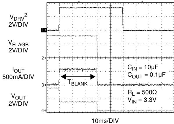
Figure 23. T<sub>BLANK</sub> Response
