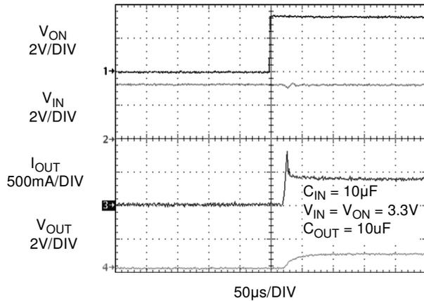
Figure 21. Current Limit Response Time (Output is loaded by 2.2Ω, C<sub>OUT</sub> = 10µF)
