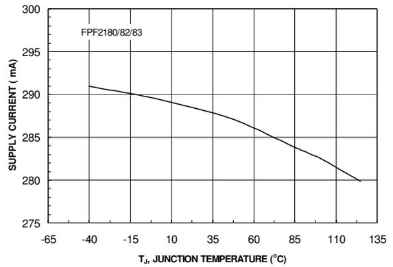
Figure 8. Current Limit vs. Temperature
