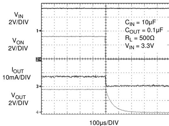
Figure 17.  $T_{OFF}$  Response
