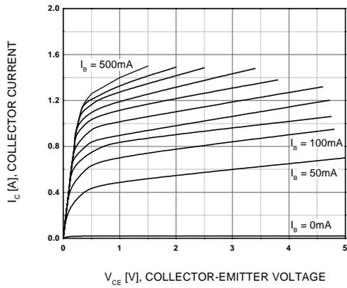
Figure 1. Static Characteristic
