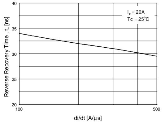
Figure 4. Typical Reverse Recovery Time vs. di/dt
