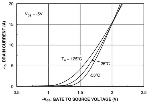
Figure 5. Transfer Characteristics.
