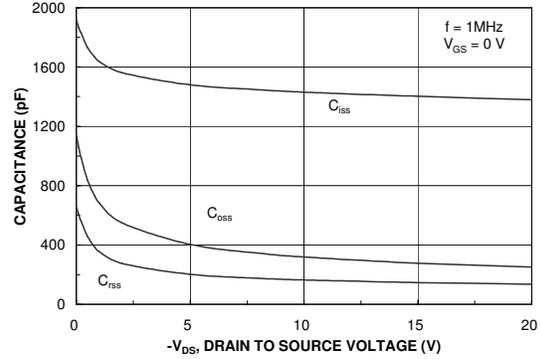
Figure 8. Capacitance Characteristics.
