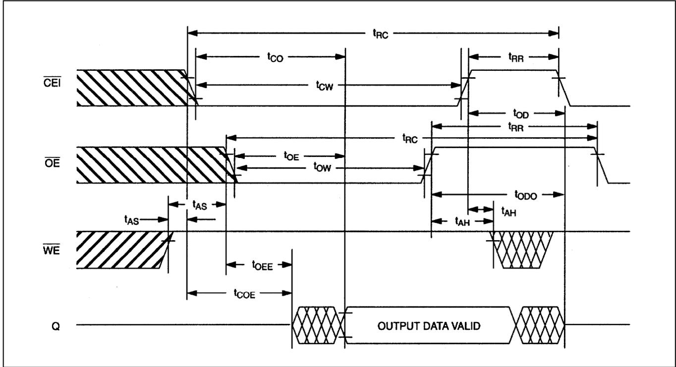
Figure 9. Timing Diagram: Write Cycle to Time Chip ROM/RAM =  $V_{CC0}$
