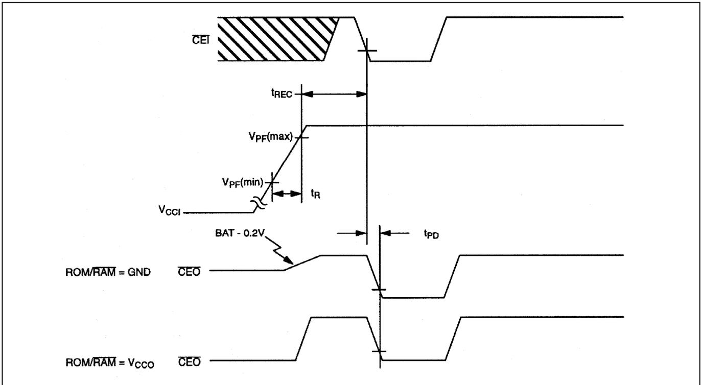
Figure 12. 5V Power-Down Condition
