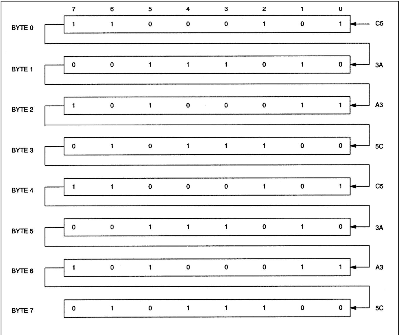
**Note:** The pattern recognition in Hex is C5, 3A, A3, 5C, C5, 3A, A3, 5C. The odds of this pattern being accidentally duplicated and causing inadvertent entry to the Phantom Time Chip are less than 1 in  $10^{19}$ .
