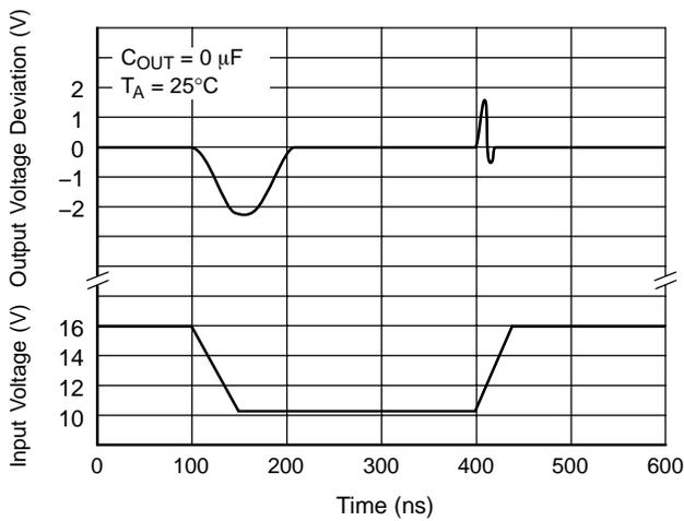
Figure 16. Regulator 1 Line Transient Response
