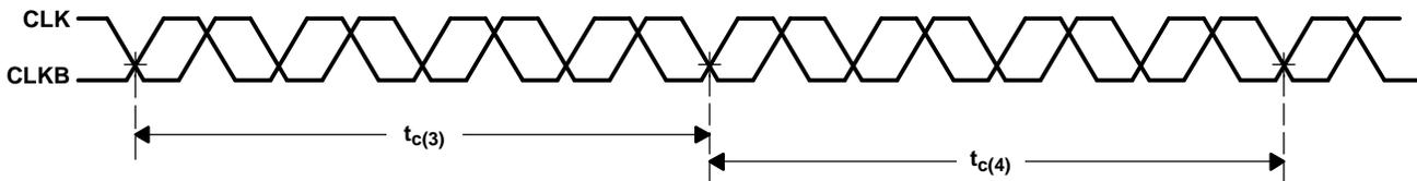
Cycle-to-cycle jitter =  $|t_{c(3)} - t_{c(4)}|$  over 10000 consecutive cycles
