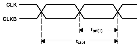
Duty cycle =  $(t_{pd(1)} / t_{c(5)})$
