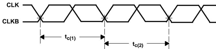
Cycle-to-cycle jitter =  $|t_{c(1)} - t_{c(2)}|$  over 10000 consecutive cycles
