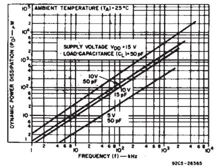
Fig. 10 - Typical dynamic power dissipation vs. frequency.
