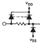
\*ALL INPUTS PROTECTED BY CMOS PROTECTION NETWORK
