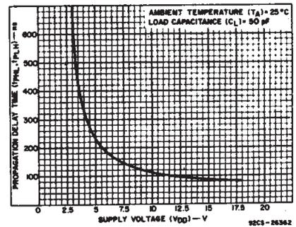
Fig. 5 - Typical propagation delay (D<sub>n</sub> to Q<sub>m</sub>) vs. supply voltage.
