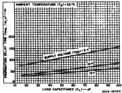
Fig. 6 - Typical propagation delay (E<sub>I</sub> to G<sub>S</sub>, E<sub>I</sub> to E<sub>O</sub>) vs. load capacitance.
