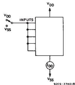
Fig. 14 - Quiescent device current test circuit.
