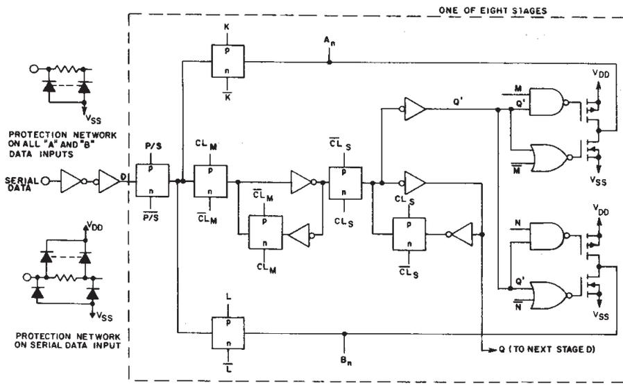
Fig. 11 - Register stage logic diagram (1 of 8 stages).
