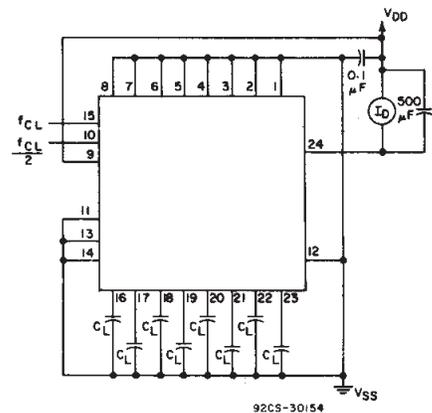
Fig. 13 - Dynamic power dissipation test circuit.
