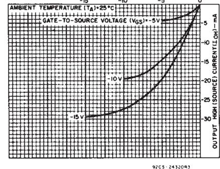
Fig. 7 - Typical output high (source) current characteristics.
