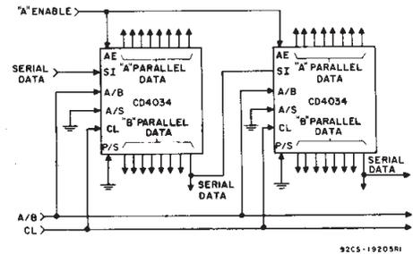
Fig. 18 — 16-bit serial in/gated parallel out register.
