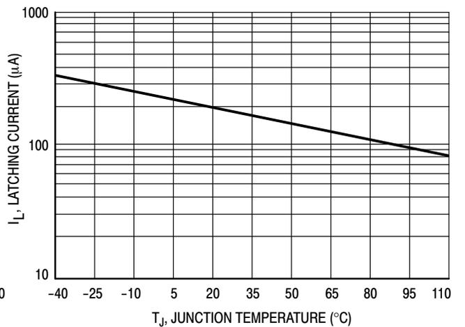
Figure 6. Typical Latching Current versus Junction Temperature
