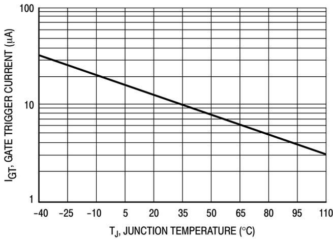
Figure 3. Typical Gate Trigger Current versus Junction Temperature
