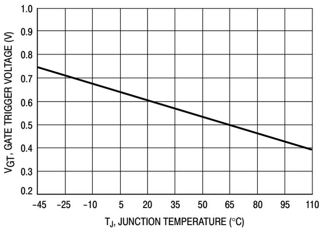
Figure 5. Typical Gate Trigger Voltage versus Junction Temperature
