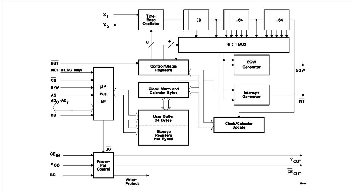
standard CMOS SRAM nonvolatile during power-fail conditions. During power-fail, the bq4285E/L automatically write-protects the external SRAM and provides a  $V_{CC}$  output sourced from the clock backup battery.
