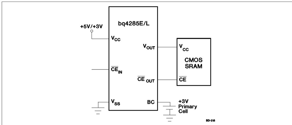
Figure 4. External RAM Hookup to the bq4285E/L RTC
