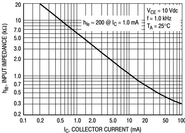
Figure 17. Input Impedance
