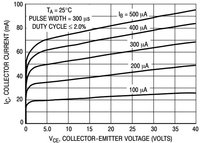
Figure 10. Collector Characteristics
