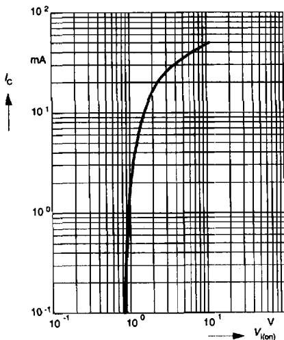
**Collector-Emitter Saturation Voltage**
